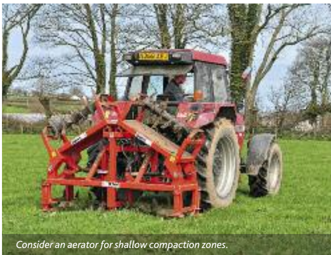
Use a grassland subsoiler which is capable of going down to 28-30cm (10-12in) but adjust depth so that it only works at 2cm below the compaction zone.
